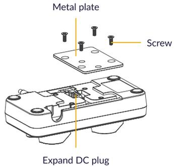
1 Remove the screws and the metal plate.
