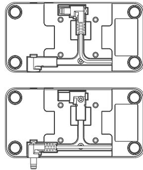
2 Take out the expand DC plug and put it as shown.
