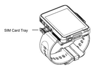
Step 1: Power off the terminal, then pull out the SIM card tray;
