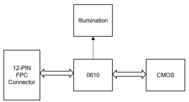
The engine connected with the host via the 12-pin FPC cable. For more details about the 12-pin FPC cable, please see **12-pin FPC** in Chapter 4.
